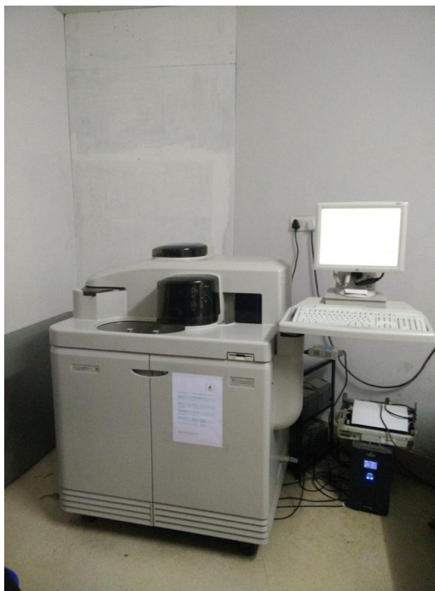
Figure 24: Photograph of chemiluminescence machine used for thyroid function tests
