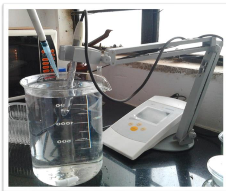
Fig 10:-Photograph showing pH meter with buffer solution
