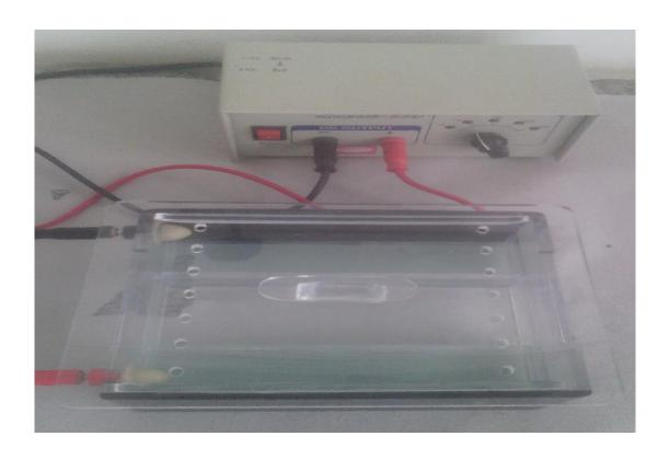
Figure 10 Gel electrophoresis apparatus
