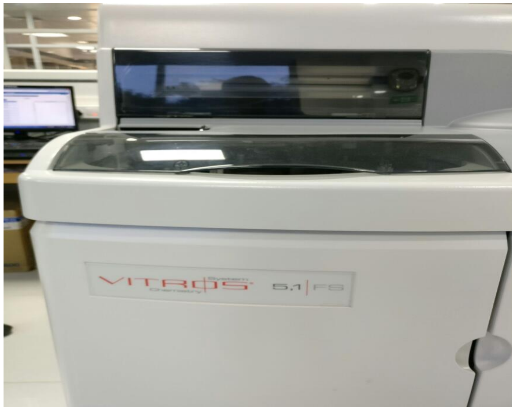
FIGURE 1 : VITROS , a machine which utilizes indirect ion-specific electrode potentiometry for sodium determination
