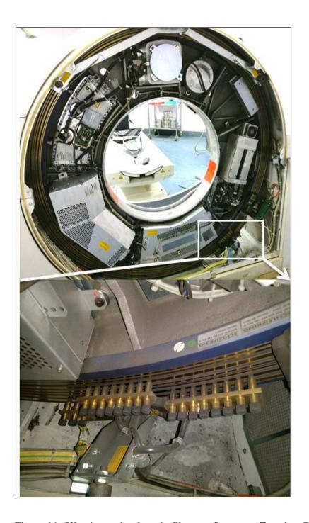
Figure 11. Slip-ring technology in Siemens Somatom Emotion CT scanner
