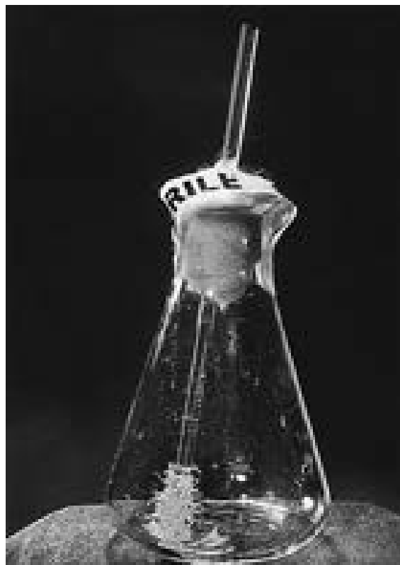
Figure 1.2 Flask for defibrinating 10–50 ml of blood. The glass rod has had some small pieces of drawn-out glass capillary fused to its lower end.
