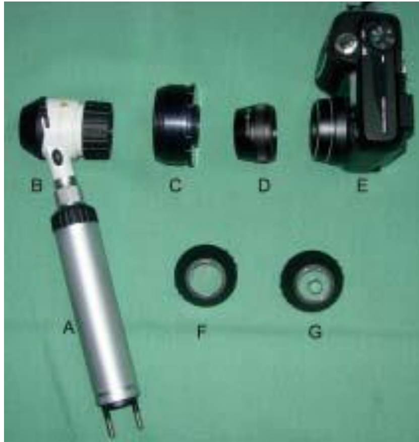
Figure 7: DELTA 20, a dermoscope with camera attachable facility. A, rechargeable handle; B, hand-piece; C, connector ring; D, photo-adaptor; E, camera; F, contact plate; G, small contact plate. 12
