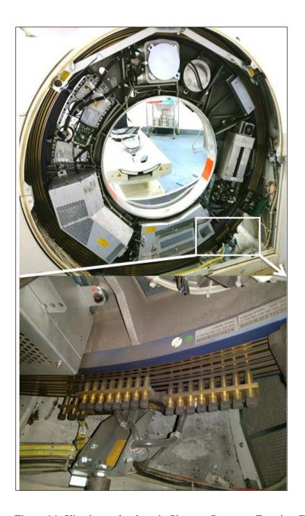
Figure 14. Slip-ring technology in Siemens Somatom Emotion CT scanner.
