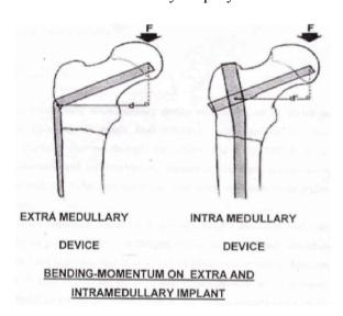
Fig. 17- Bending momentum on extra and intramedullary implant
