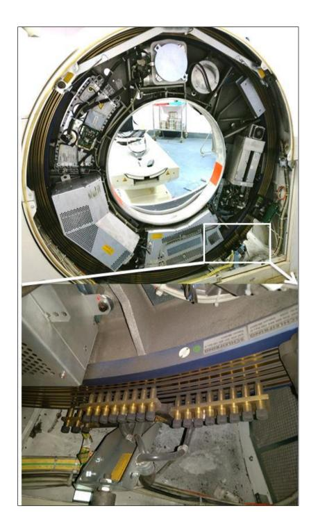
Figure 8. Slip-ring technology in Siemens Somatom Emotion CT scanner
