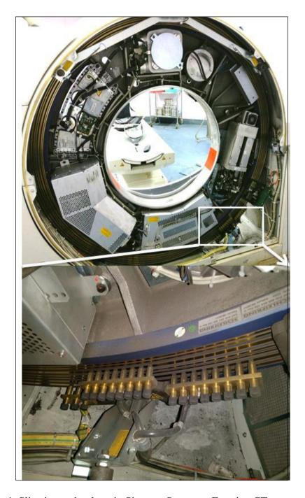
Figure 1. Slip-ring technology in Siemens Somatom Emotion CT scanner
