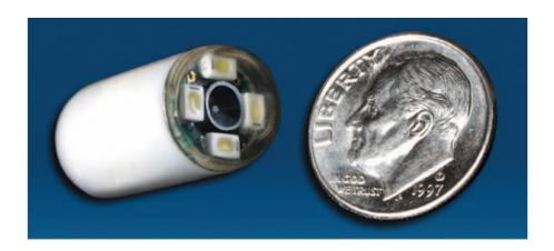
Figure 15 Capsule used in capsule endoscopy
