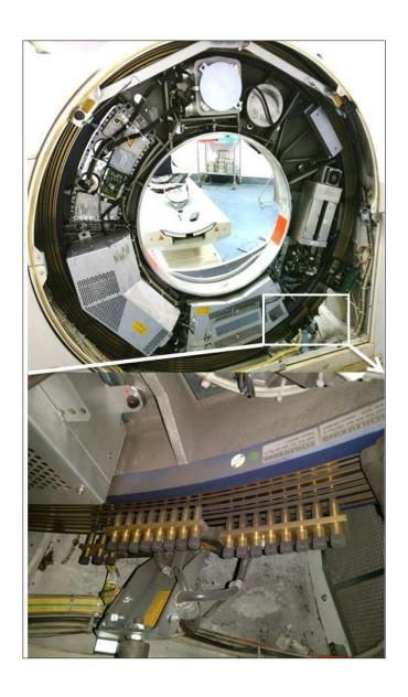
Figure 16 Slip-ring technology in Siemens Somatom Emotion CT scanner
