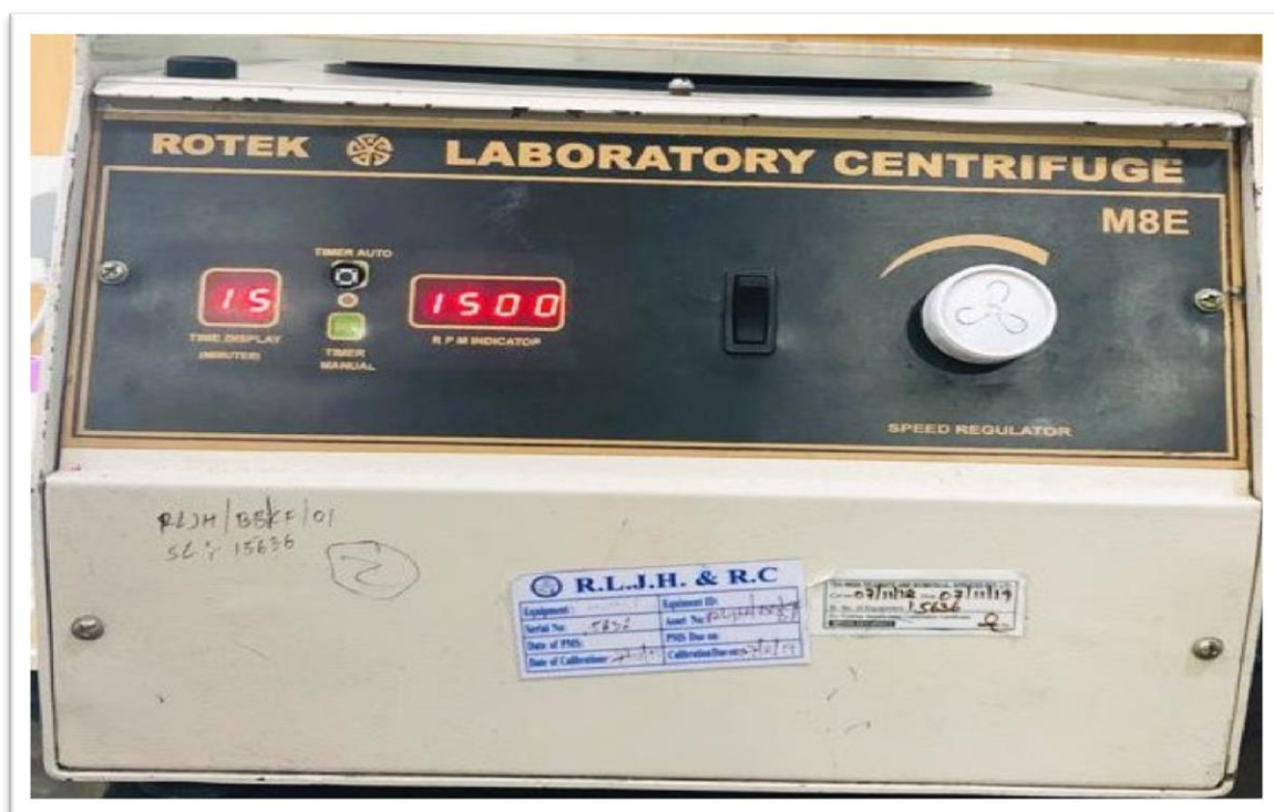
CENTRIFUGE FOR PRP SEPARATION WITH TIMER : FRONT VIEW
