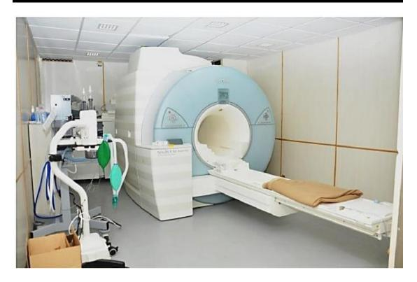
Figure 12: Siemens Magnetom Avanto® 1.5 T MRI scanner.
