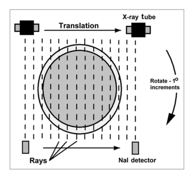
**Figure 12: X-ray transmission measurements.** Measurements are obtained at many points during translation motion of tube and detector. x-Ray path corresponding to each measurement is designated a ray, and set of rays measured during translation is designated a view. Views are collected at many angles (in 1° increments in this example) to acquire sufficient data for image reconstruction.
