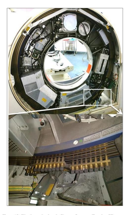
Figure 13: Slip-ring technology in Siemens Somatom Emotion CT scanner
