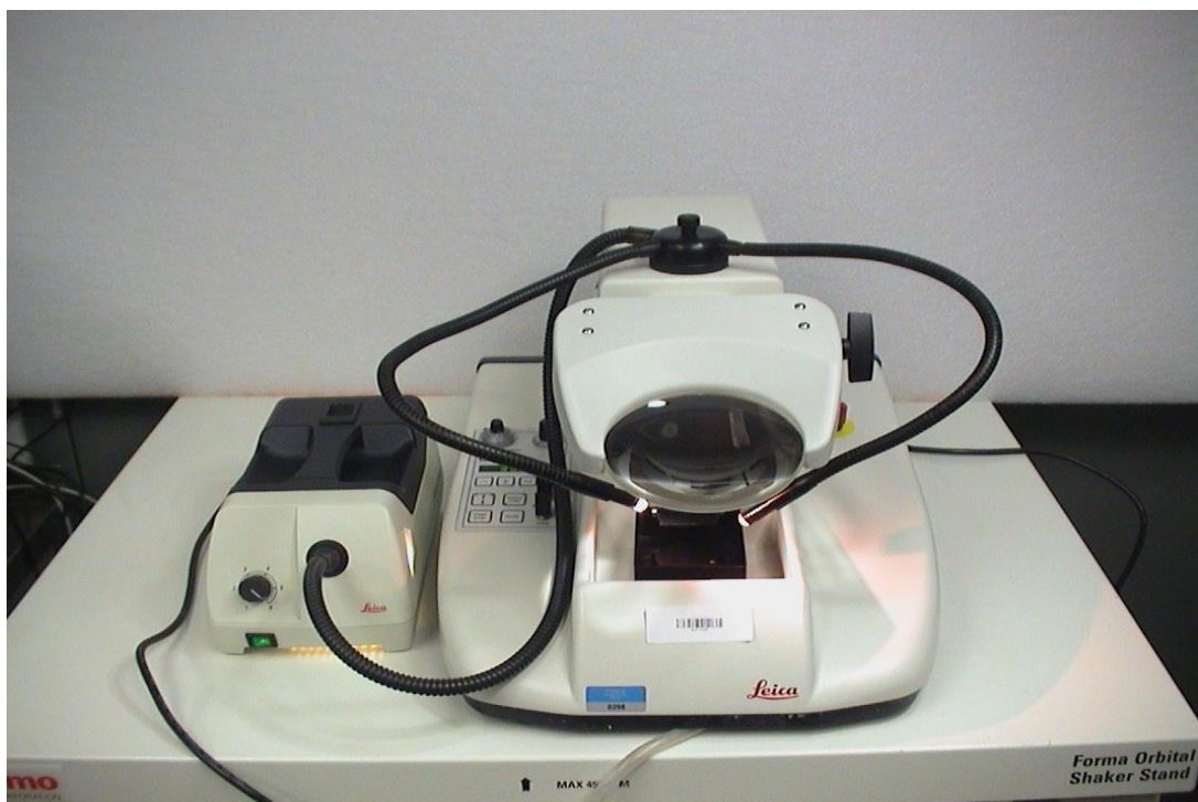
Figure 20: Vibratome microtome (Leica VT 1000 S) used to cut 150 \mu thick sections for Golgi-Cox staining to trace hippocampal CA3 pyramidal neurons-Image captured in Sectioning and staining lab, Department of Neurophysiology, NIMHANS, Bengaluru.
