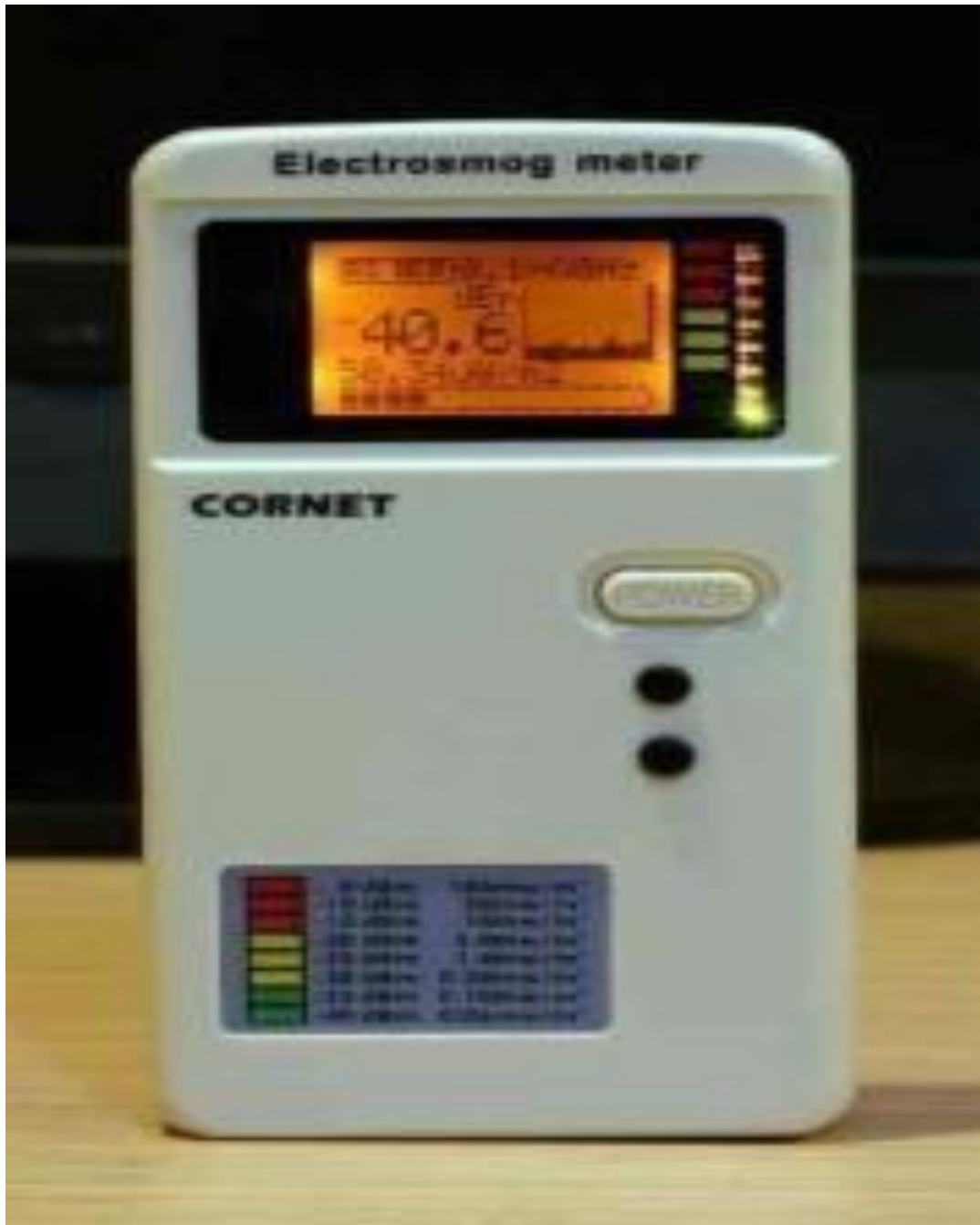
Figure 12: Radiation frequency meter (Cornet Microsystems-ED 178 electrosmog meter) – Image captured in central animal house, Sri Devaraj Urs Medical College, Kolar, Karnataka.
