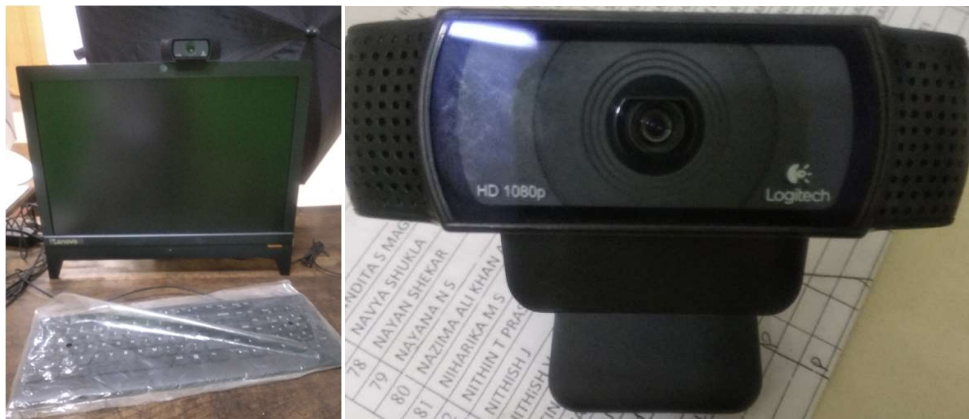
Logitech C920 webcam 1080p resolution, 30fps.
