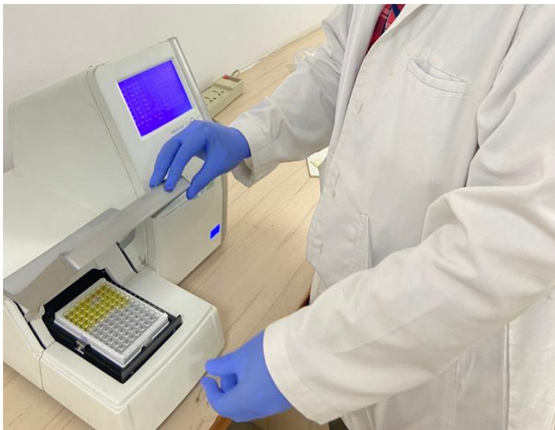
Figure 21: Image represents yellow color was measured at 450 nm. ELISA reader (Rayto, RT-6100 microplate reader)- figure captured in research laboratory, Department of Microbiology, SDUMC, Tamaka, Kolar.
