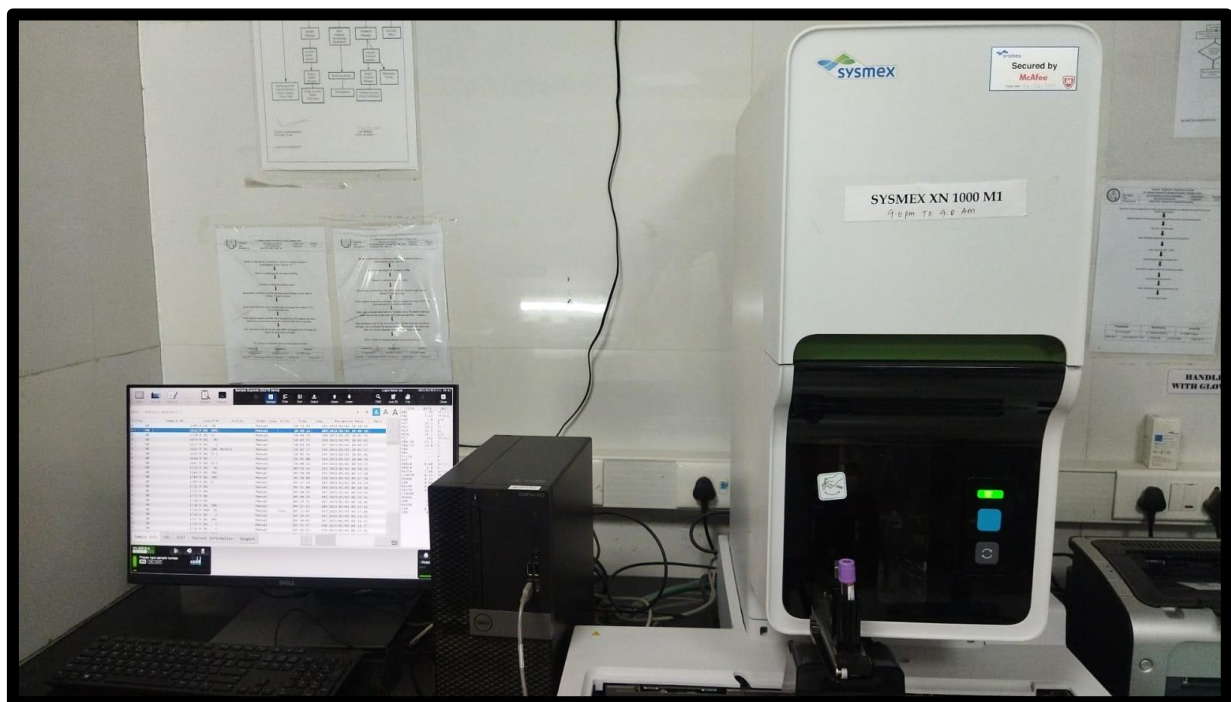
Figure 27: platelet counting machine
