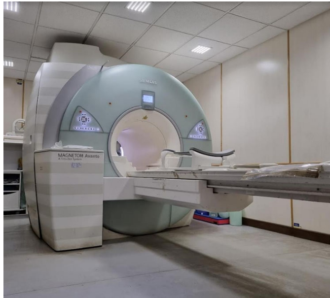
Figure 17: 1.5 Tesla, 18 channel, MR Scanner (Siemens® Magnetom Avanto®)
