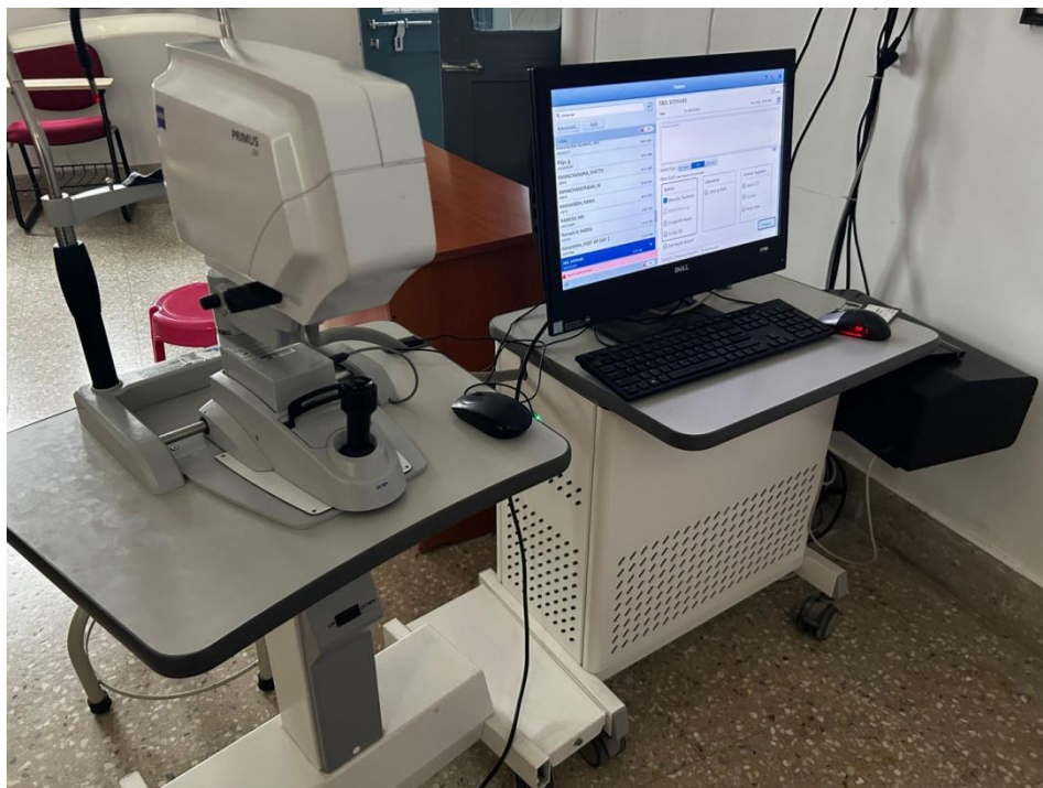
Figure 10: The PRIMUS 200 OCT system with computer display.
